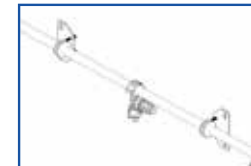
Installs Boom Mounting Plates to Boom Assembly
